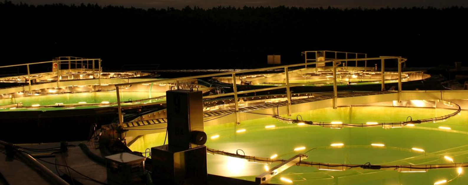
Setup of the lighting system to simulate skyglow at the LakeLab.
