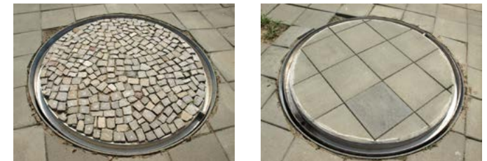
> Weighing lysimeters with different paving materials.
