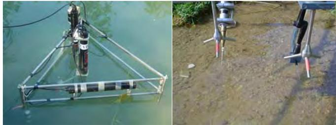
**Figure 1:** (Left) The two eddy correlation systems mounted next to each other in the measurement site. (Right) A close up of the two systems.
