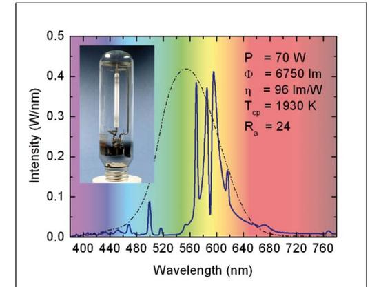
Spectrum of a high-pressure sodium lamp (solid line, OSRAM Vialox 70 W NAV(SON)-T) compared to the standard sensitivity of the human eye (dash-dotted line), with power  $P$ , luminous flux  $\Phi$ , efficiency  $\eta$ , colour temperature  $T_{cp}$  and colour rendering  $R_a$ .
