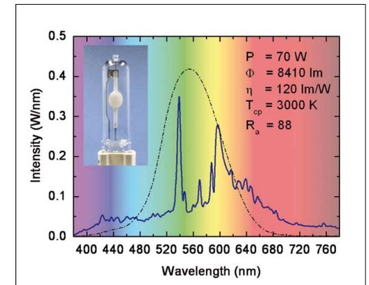
Specifications of a metal halide lamp (OSRAM Powerball HCI-T 70 W / WDL) compared to the standard sensitivity of the human eye (dash-dotted line).
